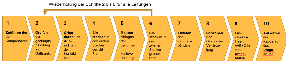
Figure 14: Process chain for assembling the wiring harness
