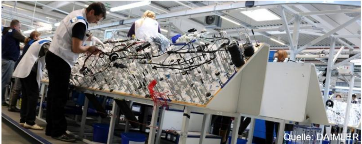
Figure 2: Manual final assembly of wiring harnesses on moulding boards
