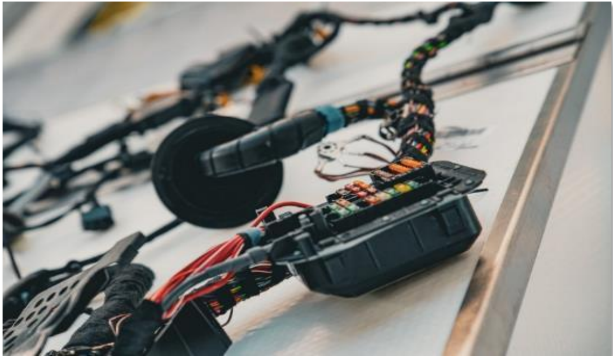
Figure 1: Example wiring set with integrated fuse box
